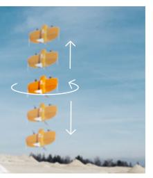
As a VTOL drone, WingtraOne can fly in two modes: hover and forward flight. While hovering, WingtraOne can be manually operated to fly in any direction like a helicopter: up and down, back and forward and to both sides.
